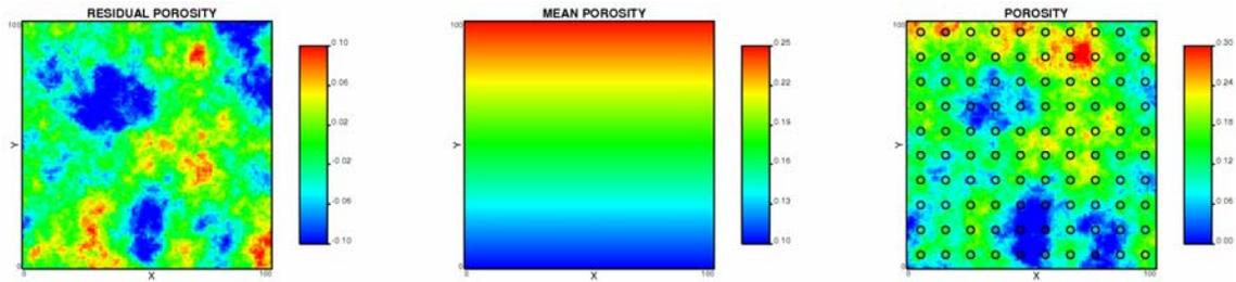
**Figure 1:** The construction of a non-stationary porosity random function showing the residuals (left), locally varying mean (middle), and resulting porosity variable (right). The dark circles represent sample data locations.
