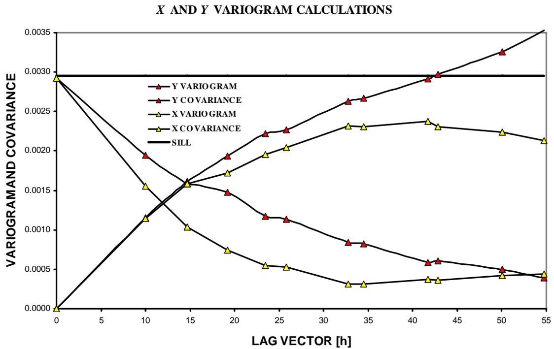
**Figure 2:** The X and Y direction experimental variograms for the porosity sample data set constructed in Figure 1.
